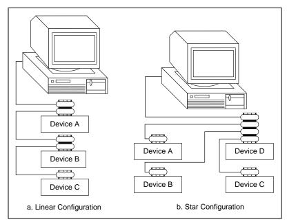
Figure 1-1. Linear and Star System Configuration
