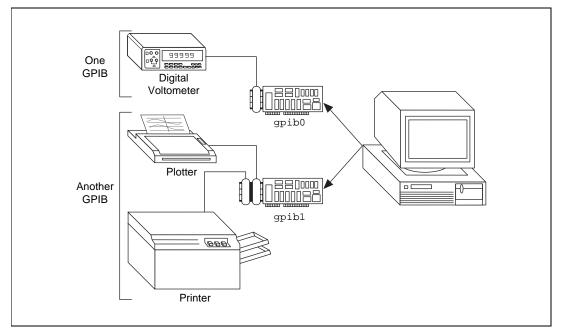
Figure 1-2. Example of Multiboard System Configuration
